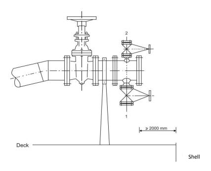
Connection for depositing residues. Connection pursuant to standards:
