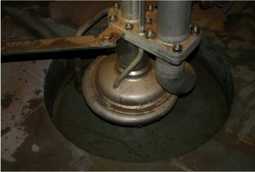
Figure 3: Photo from a well in bottom of double hull tank in barge (Photo provided with memo [14])
